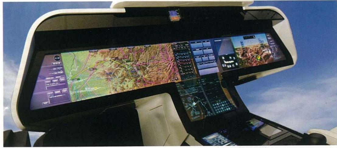
The flightdeck would provide the functionality of multiple displays via a single touchscreen, tailored for individual pilots
